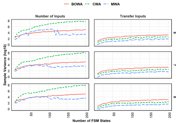
Fig. 10: Averages of sample variance of the number of inputs and number of transfer inputs of state identification sequences across varying numbers of inputs/outputs and algorithms given in \log_{10} scale. Higher variance reflects increased structural diversity in the state-transitions of the synthetic FSMs.
