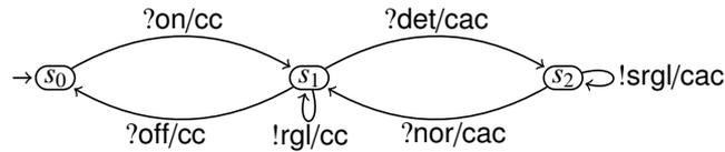
Figure 2: IOFTS of the cruise controller.
