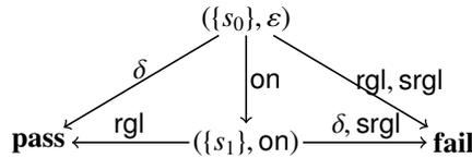
Figure 5: A test case of the cruise controller.
