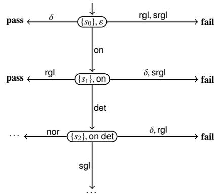
Figure 10: Spinal test suite of the cruise controller
