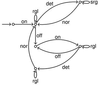
Figure 11: A faulty implementation of the cruise controller with control avoidance.
